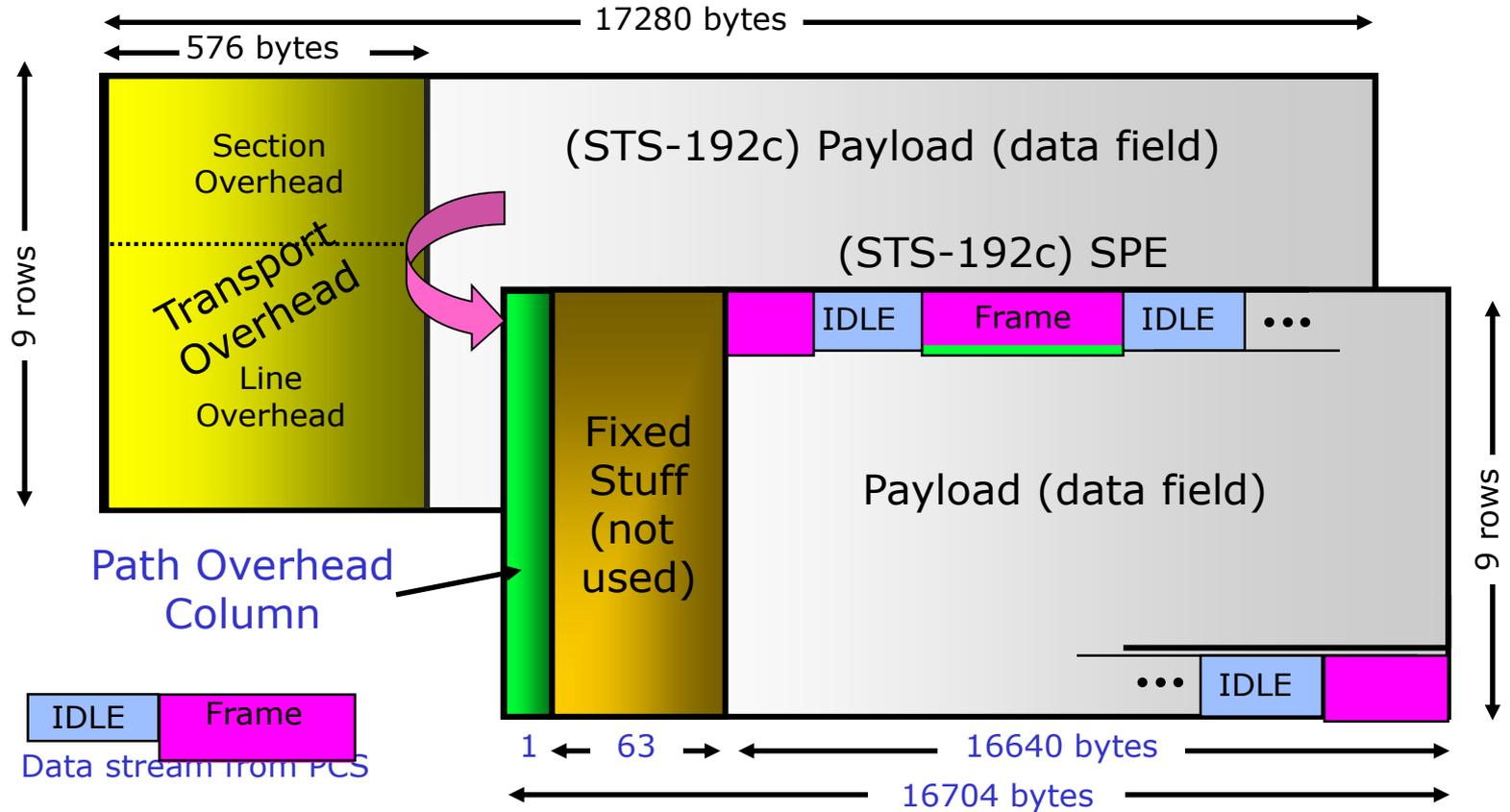
STS-192c = Synchronous Transport Signal – of level 192, c = concatenated
